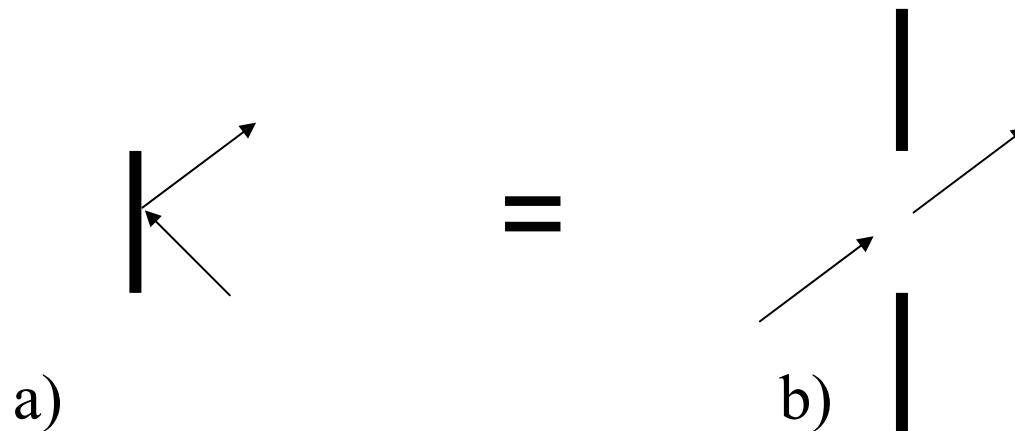
Reflection from a surface (a) is equivalent to transmission through an aperture (b) with same size and shape, surrounded by a rigid baffle
